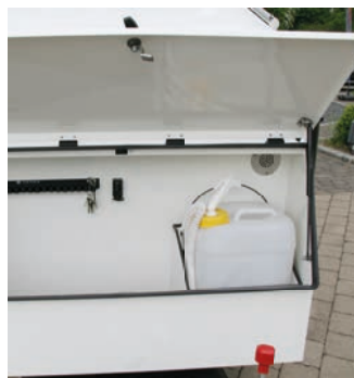
• Front storage box with water tank
